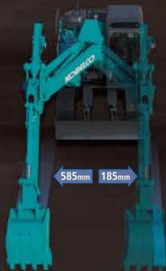
Standard equipment includes an offset boom, and a dozer blade makes swift work of excavation next to walls or of side ditches, as well as refilling.
