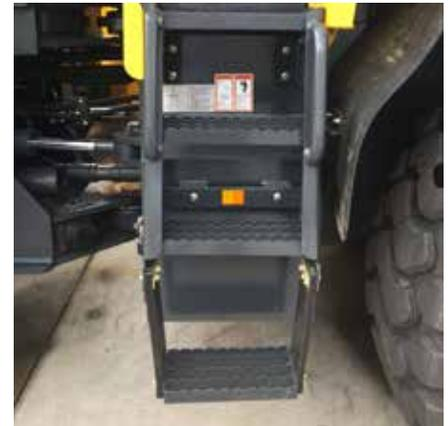
Access to the front of the cab by the operator or service person is a new feature. The same anti-slip bars used on the egress steps are used here for maximum anti-slip protection.
