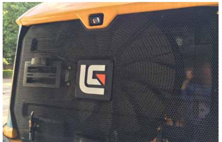
All-around visibility is supported by a rear-view camera acting as an extra eye on the jobsite.
