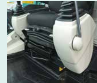
Seat suspension absorbs vibration
